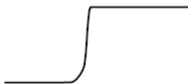
Signal with a short ground lead
