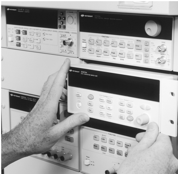
Low-cost switching system for automated testing
